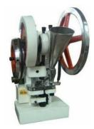
A tablet press can be used to create tablets from pharmaceuticals, nutraceuticals, cleaning products, industrial pellets, and cosmetic products. Granulated powder material is metered into a cavity made by two punches and a die, and then the material is fused together by applying high power to the punches, which is how tablets are made.[17]
