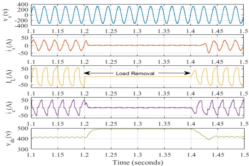
Fig. 6 Dynamic response of single phase grid interfaced solar PV system under fixed solar irradiance level feeding unbalanced nonlinear load.
