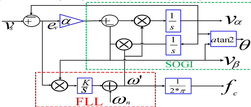
Fig. 2 Structure of SOGI-FLL for synchronization
