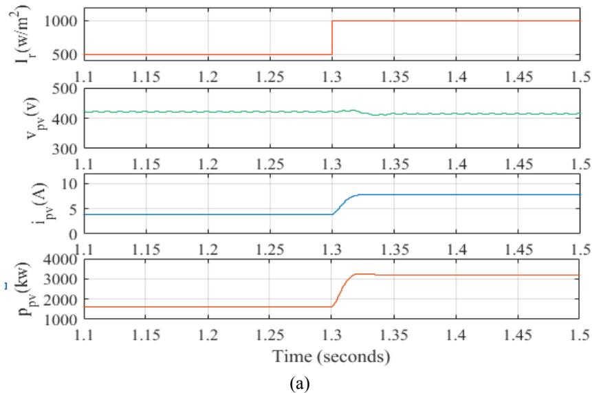
Fig. 5(a) and (b) represents dynamic response of single phase grid interfaced system under change in solar irradiance feeding balanced load. Fig. 5(a) shows the change in solar irradiance from  $500 \text{ w/m}^2$  to  $1000 \text{ w/m}^2$  at  $t=1.3\text{s}$ . During the change in solar irradiance level, the PV current and PV power is increased. Fig. 5(b) shows the dynamic response of
