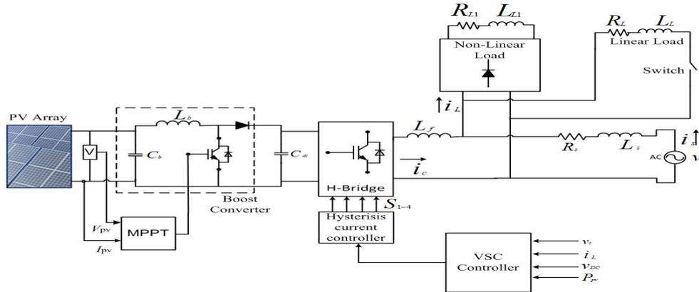
Fig. 1 Structure of 1-phase grid connected PV system
