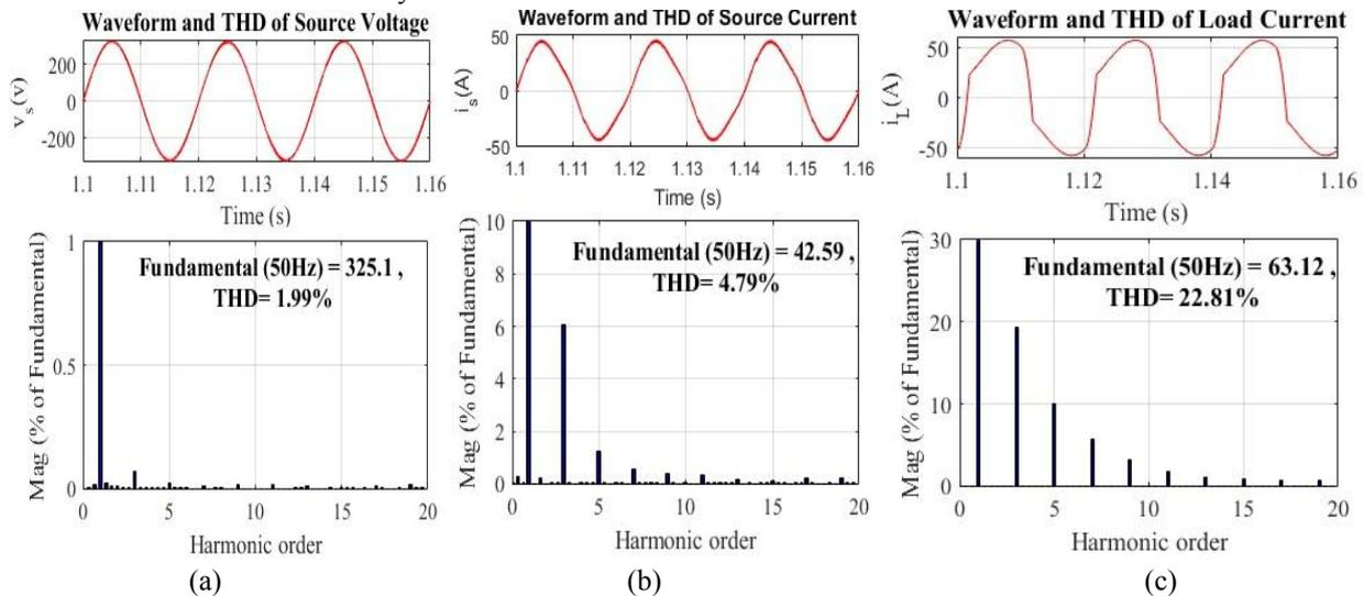
Fig. 7(a)-(c) Harmonic analysis of source voltage, source current and load current
