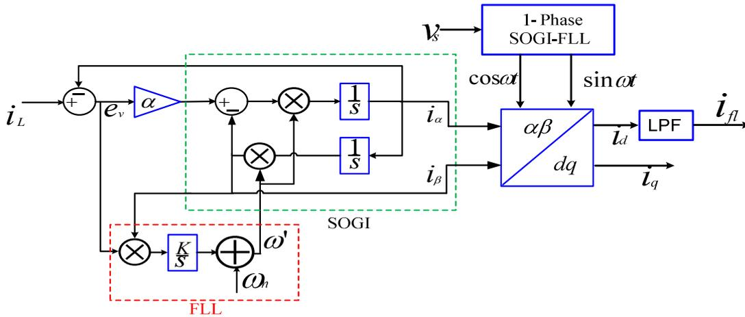
Fig. 3 SOGI-FLL control algorithm
