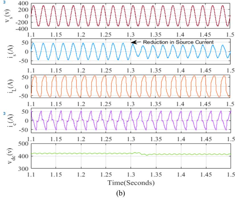
Fig. 5(a) and (b) represents dynamic response of single phase grid interfaced system under change in solar irradiance feeding balanced load
