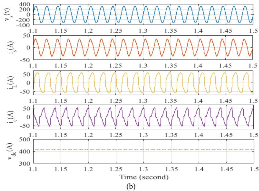
Fig. 4(a) and (b) Steady state response of the proposed system under fixed solar irradiance feeding balanced nonlinear load
