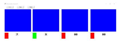
After vehicle detection on the basis of vehicle count time will be set as per the traffic. After counting number of vehicle Calculate time required to traffic signal light ON/OFF time period and send command to hardware as per time schedule. With the timer controller, we can control heavy traffic congestion in just couple of seconds (100 seconds).
