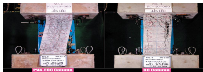
Figure c: Cracking Phenomenon in concrete
