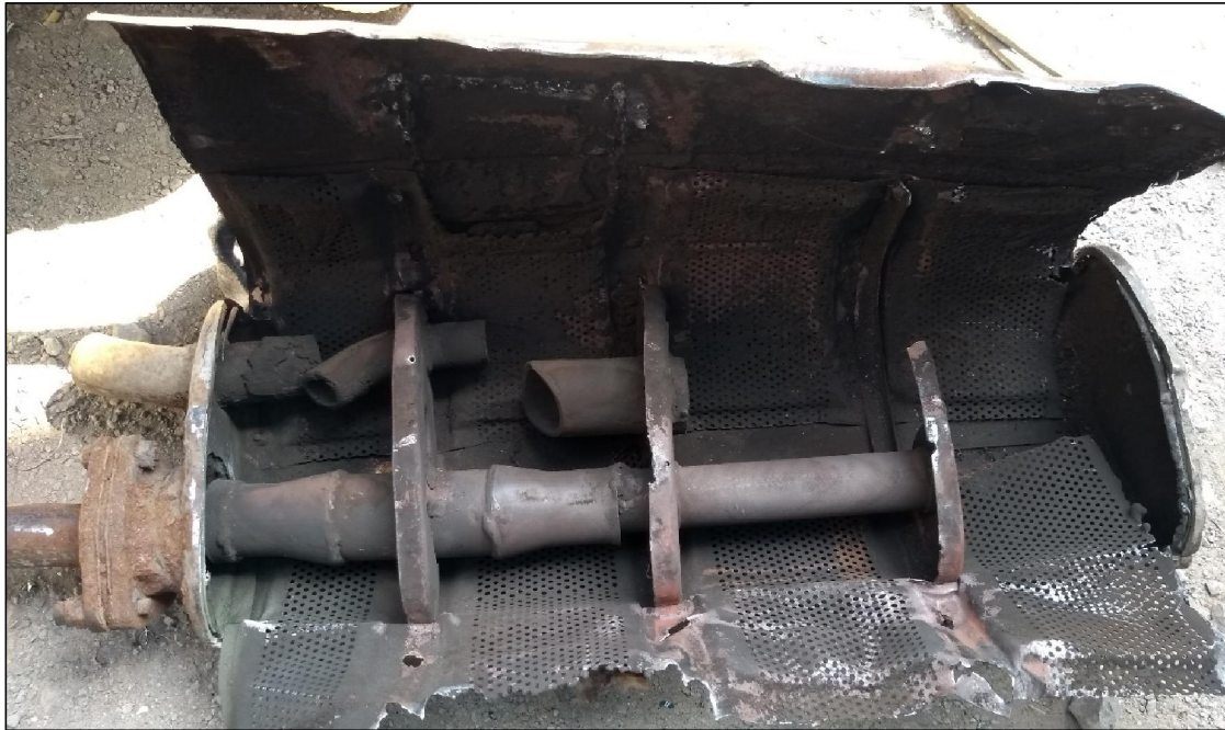
Fig. Existing 3 wheeler muffler with open section view
