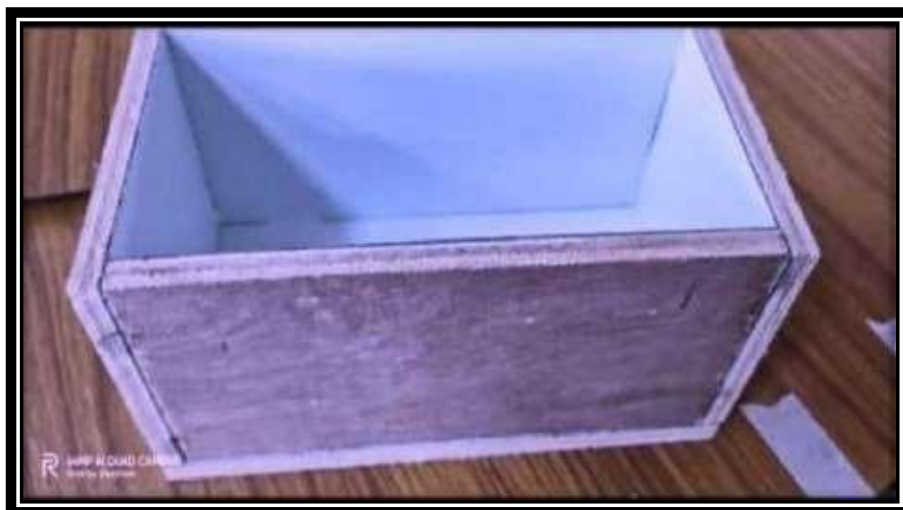
Fig 3: Mould of Size 19mmX19mmX9mm
