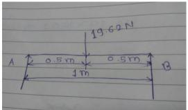
As we know for shear force equation Sum of horizontal forces,  $\Sigma$  Fx= 0,  $\Sigma$  Fy = 0 Ra + Rb - W = 0  $\therefore$  Ra + Rb = 19.62 NAL = 0 Moment about A and B = 0AR = 9.81 N  $Ma = (Rbx 1) - (19.62 \times 0.5)$ CL = 9.81 N CR = -9.81 N As we know, Rb = 9.81 NBL = -9.81 N Ra + Rb = 19.62 NBR = 0 NRa = 9.81 N **Copyright to IJARSCT** DOI: 10.48175/568 www.ijarsct.co.in
