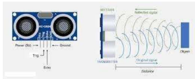
Fig.2. HC-SR04 ultrasonic sensor working
