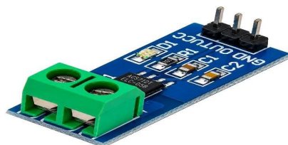
Fig. 11 — ACS712 current sensor
