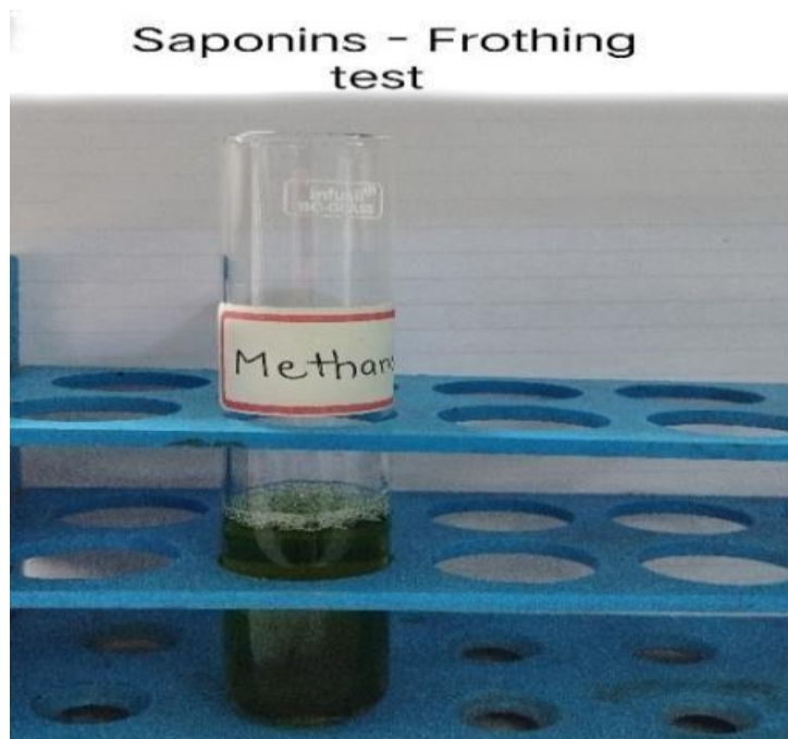
Figure 5. Saponins test (frothing test).
