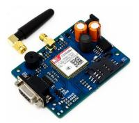
The SIM800A Quad-Band GSM/GPRS Module with RS232 Interface is a complete Quad-band GSM/GPRS solution in an LGA (Land grid array) type which can be embedded in the customer applications. SIM800A support Quad-band 850/900/1800/1900 MHz, it can transmit Voice, SMS and data information with low power consumption.
