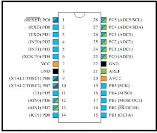
The Atmel ATmega328 is a low-power CMOS 8-bit microcontroller based on the AVR enhanced RISC architecture. By executing powerful instructions in a single clock cycle, the ATmega8A achieves throughputs close to 1MIPS per MHz. This empowers system designer to optimize the device for power consumption versus processing speed.
