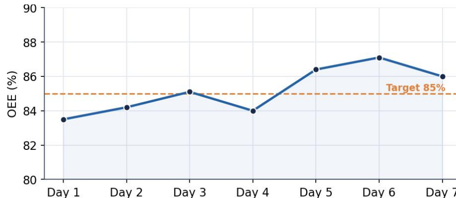
Fig. 5 Illustrative seven-day OEE trend against a target line, supporting shift-level review.
