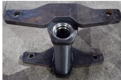
Figure 13: Actual photo of the Bogie Frame Assembly
