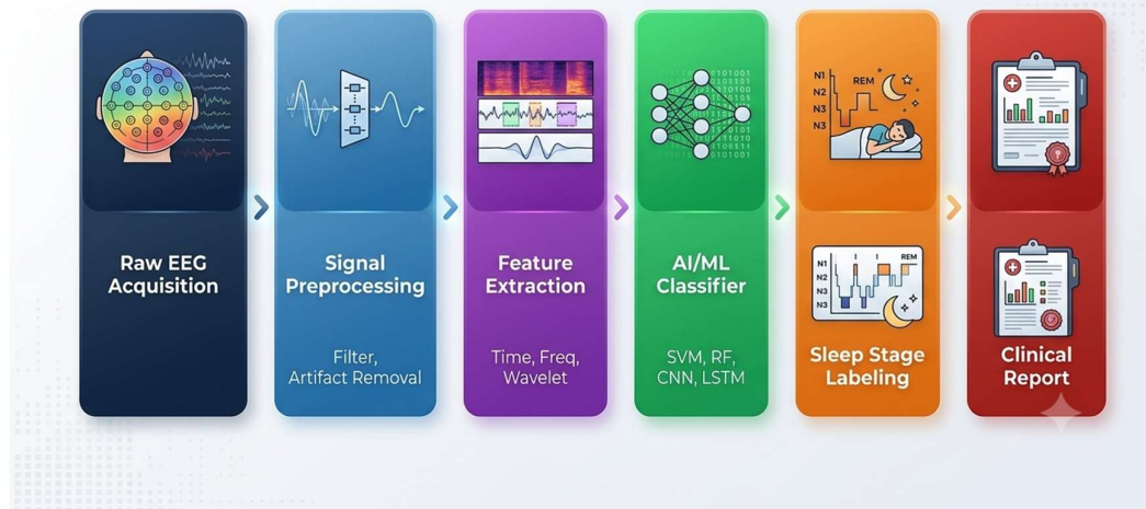
Figure 3: End-to-end AI flowchart for EEG-based sleep analysis, illustrating the sequence-wise transformation from raw bio signal acquisition to structured clinical reporting.[3]
