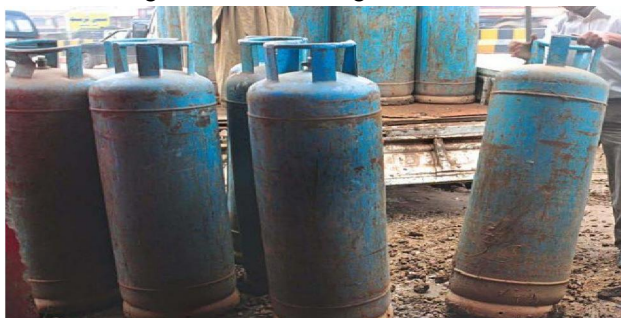
Figure 2 Improper way of handling Chlorine Cylinder
