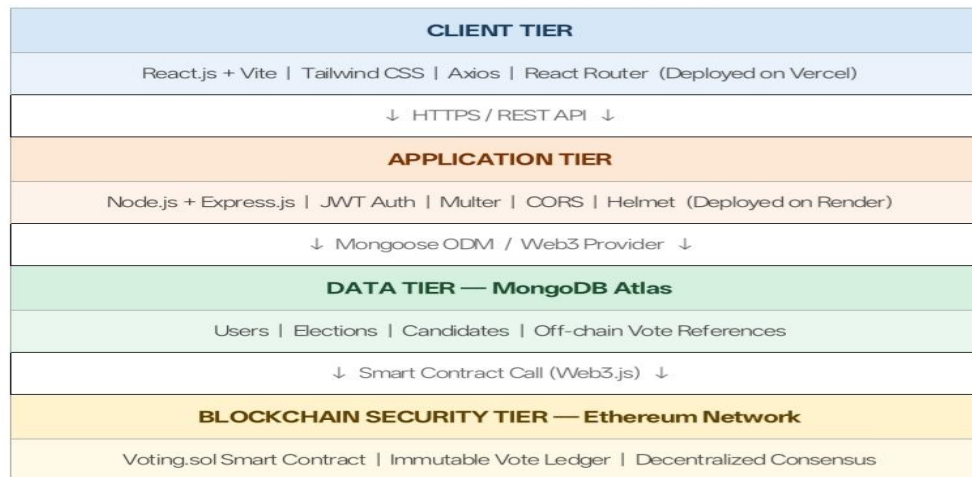
Fig. 1. High-level architecture showing the Client Tier, Application Tier, the MongoDB off-chain data store, and the Ethereum blockchain security layer connected through a smart contract interface.
