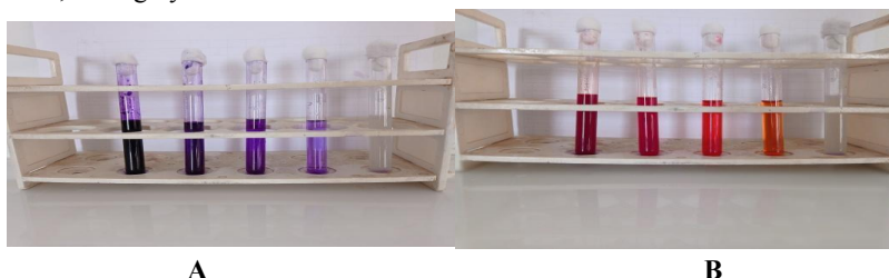
Fig 6. Biodegradation of dyes in liquid medium A) Decolorization of Crystal violet B) Decolorization of Congo red
