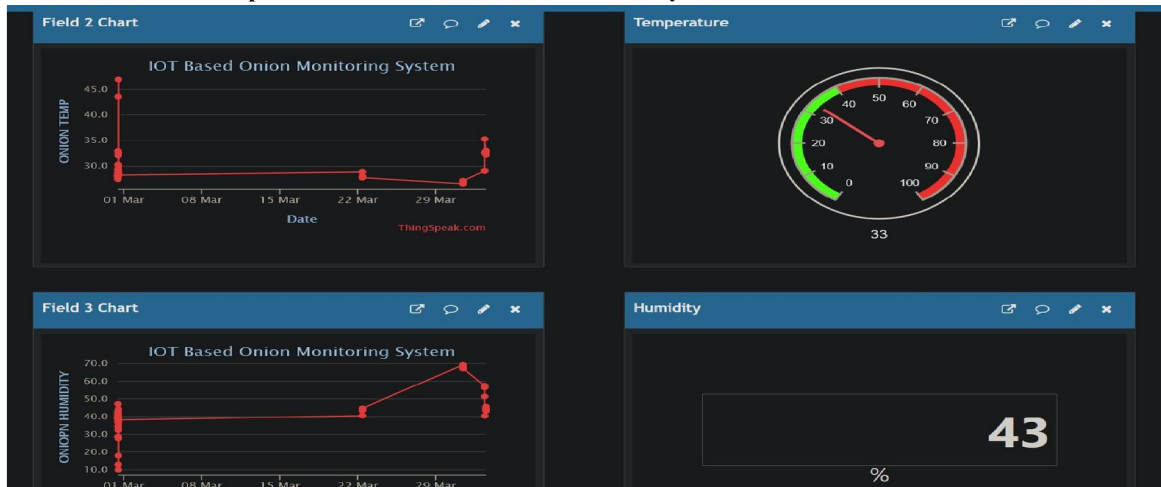
Fig. 3. ThingSpeak Field 2 Chart (Onion Temperature, °C) with gauge showing 33°C, and Field 3 Chart (Onion Humidity, %) with numeric display showing 43% — both within safe storage thresholds for March 2026.
