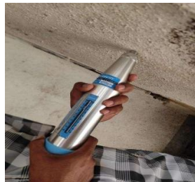
Fig.4 Rebound Hammer Test on Site
