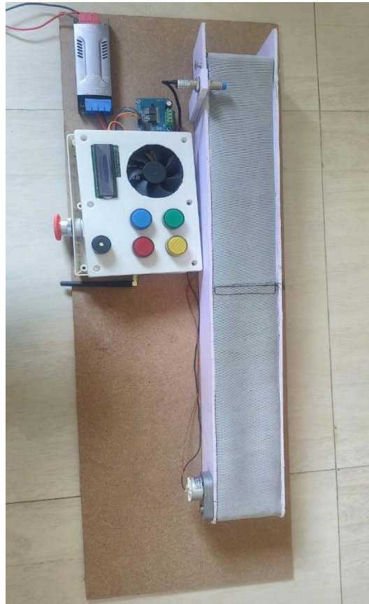
Fig. 9. Developed Prototype of LoRa-Based Wireless Conveyor Metal Sorting System
