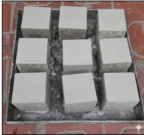
Fig 4: Concrete Test Cubes
