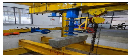
Fig.2: Flexural Testing of Reinforced Concrete Beam
