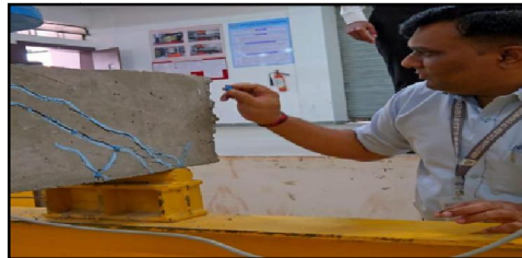
Fig.3: Analysis of Failure Pattern of Beam
