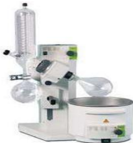
Fig No. 17: Typical photograph of Rotavapor apparatus.
