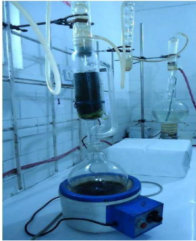
Fig.6 Schematic diagram Soxhlet Apparatus
