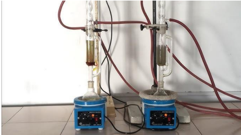
Fig 12: Soxhlet Extraction of Papaya Leaves
