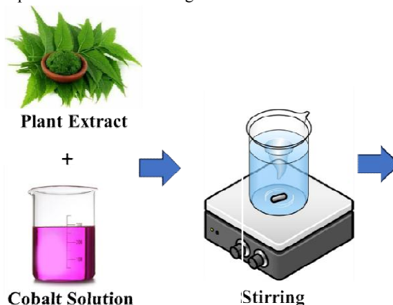
Fig. 1 Schematic representation of green synthesis of cobalt-derived material using plant extract, followed by thermal treatment to obtain the final powdered product.
