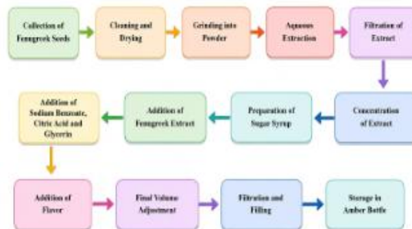
Figure 1: Step-by-step manufacturing process flowchart of fenugreek herbal syrup.
