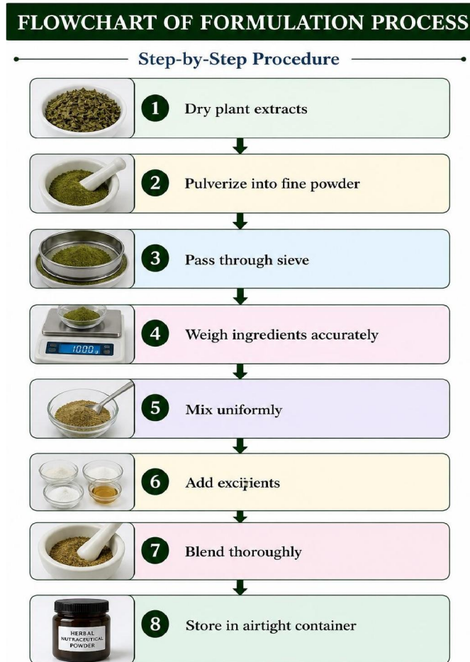
Fig. 8: Flowchart of Formulation Process
