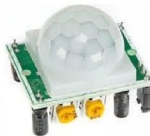
Fig 3: PIR Motion Sensor
