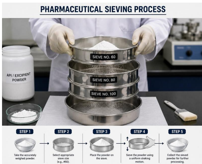
Fig. No. 8: Pharmaceutical sieving process
