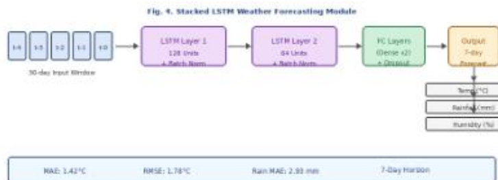
Fig. 4. Stacked LSTM Weather Forecasting Architecture
