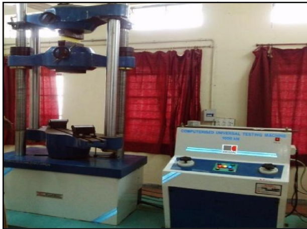
Fig. 8.1 Composite I-Beam Tensile Testing
