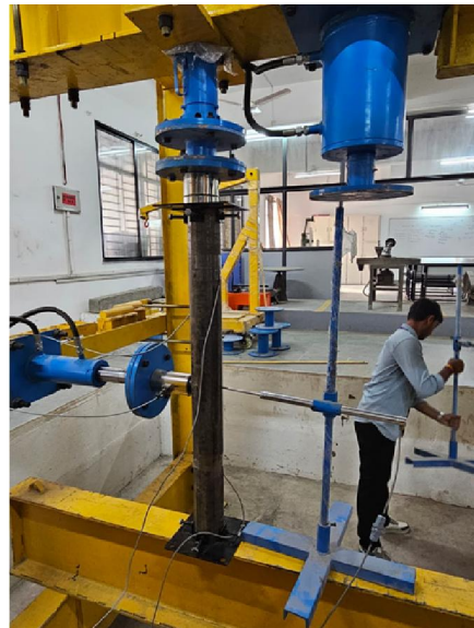
Fig 14: CFST column testing
