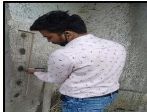
Figure 5: Rebound Hammer Testing
