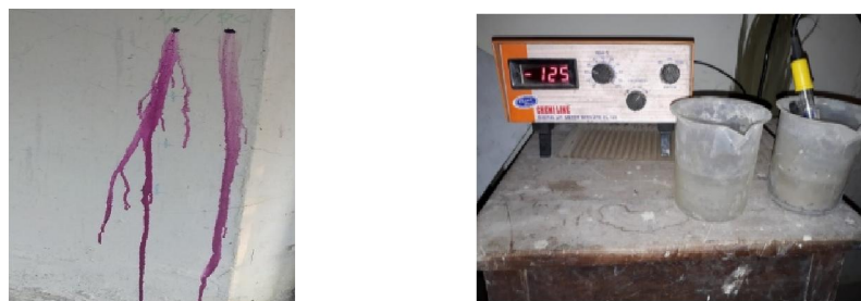
Figure 7: pH and Carbonation Test.
