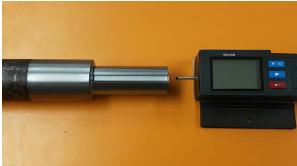
FIG. 7.1 SURFACE ROUGHNESS MEASUREMENT
