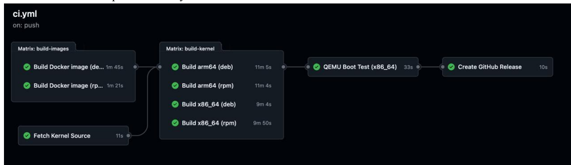
Fig. 2. Actual GitHub Actions CI/CD pipeline (ci.yml, on: push). The pipeline comprises four sequential stages. Matrix: build-images builds the DEB and RPM Docker builder images in parallel (1m 45s and 1m 21s respectively). Concurrently, Fetch Kernel Source downloads and verifies the linux-6.6.30.tar.xz tarball (11s). Once both complete, Matrix: build-kernel runs all four targets in parallel: ARM64 builds complete in approximately 11 minutes and x86_64 builds in approximately 9–10 minutes. The resulting kernel images are then validated by QEMU Boot Test (x86_64) (33s) before Create GitHub Release (10s) publishes signed packages as release assets. All stages passed.
