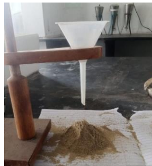
Fig no. 2 : Angle Of Repose
