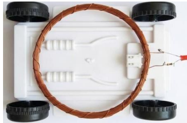
Fig 4. Wireless Receiver Panel
