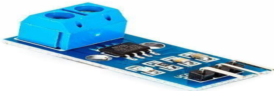
Fig..3 ACS712 5A Current Sensor
