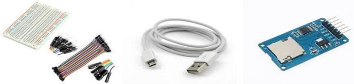
Fig. 5. Breadboard and Jumper Wires (left), Fig. 6. USB Cable for ESP32 Programming (center), Fig. 7. SD Card Module - SPI Interface (right)
