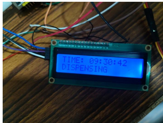
Figure 2: LCD display showing real-time system status during medicine dispensing in the proposed IoT-based adherence monitoring system.
