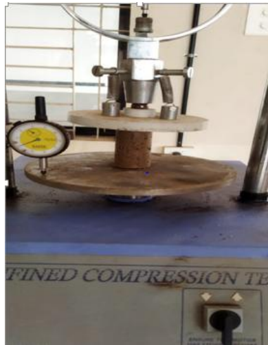
Figure 3: Unconfined Compressive Strength Test Apparatus
