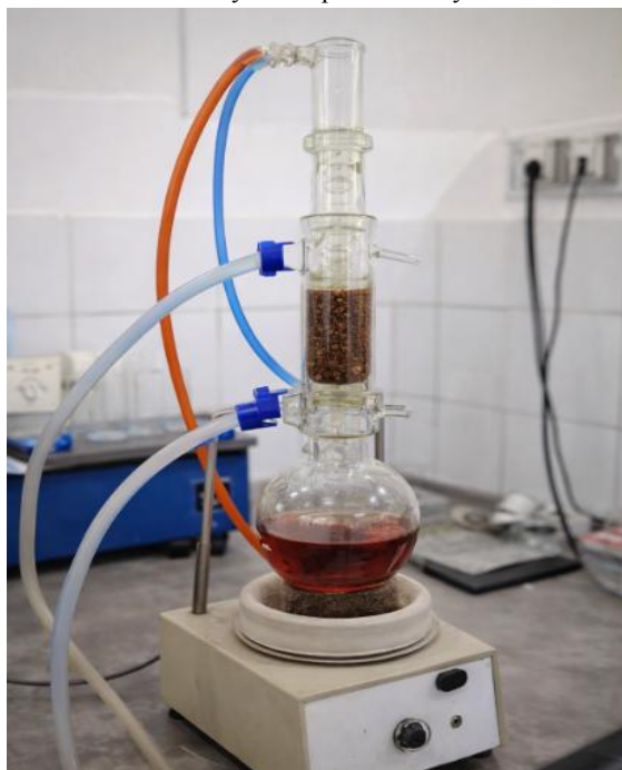
Figure 3: Soxhlet Extraction of Rubia cordifolia
