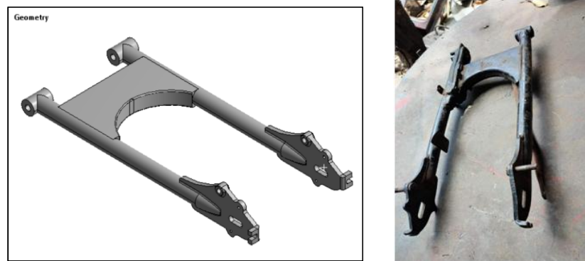
Figure 3: Geometry of swing arm
