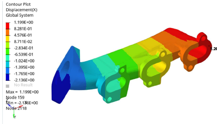
Figure 4.6 Axial displacement of exhaust manifold
