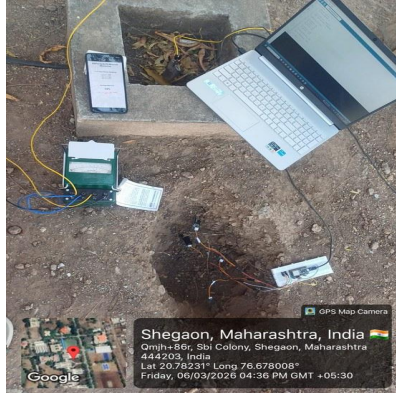
Fig. 7. Dry-pit test at Shegaon, 06/03/2026, 16:36 IST. WECO tester with 61.8 % probe arrangement [5],[6], ESP32 breadboard, laptop serial monitor, and smartphone dashboard showing 24 % moisture with LOW MOISTURE alert. Fig. 8 shows the WECO display at the dry reading, confirming the measurement falls above 5 Ω.
