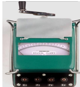
Fig. 3. WECO earth tester (61.8% fall-of-potential method, IS 3043 [5] / IEEE Std 81 [6]). Used only at calibration; removed from the monitoring loop thereafter.
