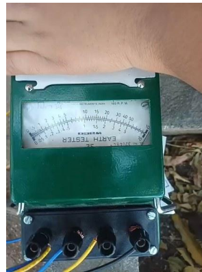
Fig. 8. WECO tester close-up during dry-pit reading. Needle position corresponds to resistance above 5 Ω (IS 3043 [5] non-compliant zone).
