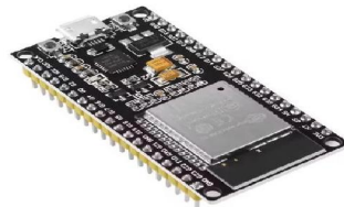
Fig. 1. ESP32 Wi-Fi microcontroller operating in softAP mode. No external Ethernet shield is required, unlike earlier monitoring designs [4].
