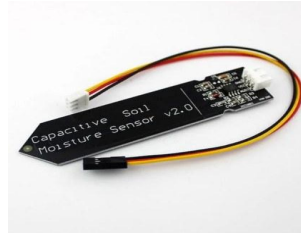
Fig. 2. Capacitive Soil Moisture Sensor v2.0. Each unit was depth-calibrated against oven-dry and saturated-soil endpoints, following the protocol of [14].
