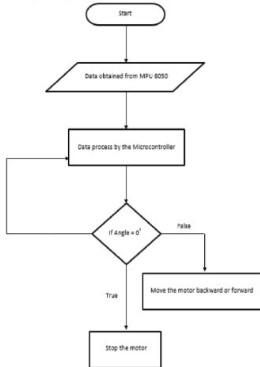
Fig. 4. Control Flow of Robot
