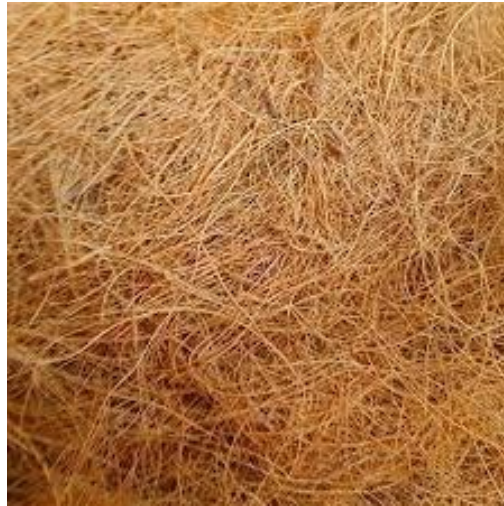
Fig. 2 Alkali-Treated Coconut Coir Fiber Mat Used as Natural Fiber Reinforcement
