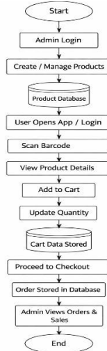
Fig. 1: AutoScan Barcode Checkout System Flow
