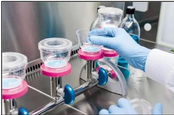
Fig 3. (a) Membrane filtration under LAF
