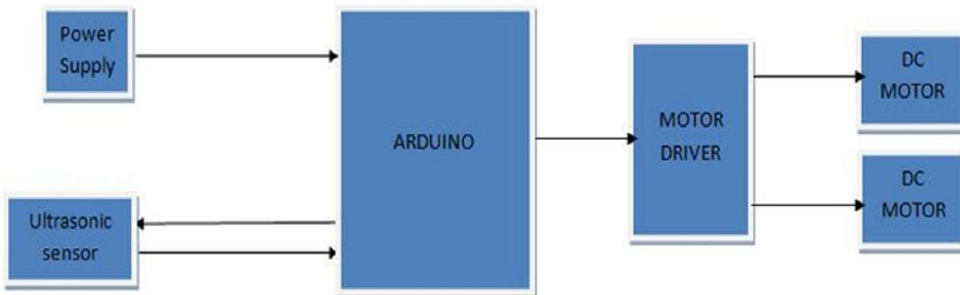
Fig 2.2:- Block Diagram
